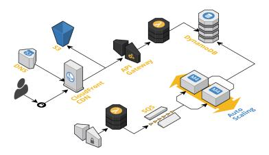
Figure 2: Overview of our highly cost efficient cloud architecture utilising AWS to provide sufficient computational resources to execute our complex trading models.
